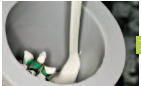
The investment ring was filled with a steady stream of vibrated investment.
