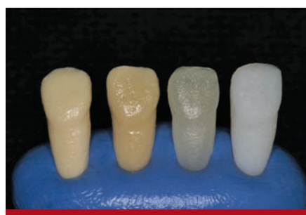
Figure 6 The technician tests the porcelain system by making and firing sample tabs in the laboratory. The sample tabs (left to right) are made of: opacous dentin, dentin, translucent, and enamel.
