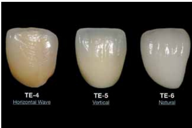
Figure 18: A second set of fabricated zirconia samples demonstrate such surface textures as horizontal waves (TE-4), vertical waves (TE-5), and natural appearance (TE-6).
