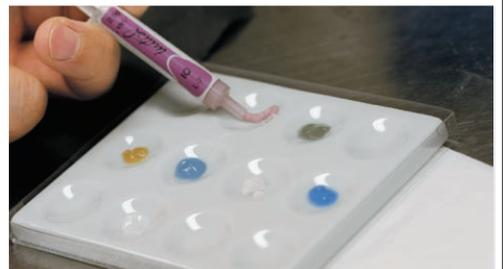
**Fig. F** Luster Pastes are dispensed from syringes and are thicker than glaze.
